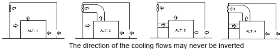
For alternatives 2 & 4 fan capacity should match the compressor fan capacity at a pressure head equal to the pressure drop across the cooling ducts.
