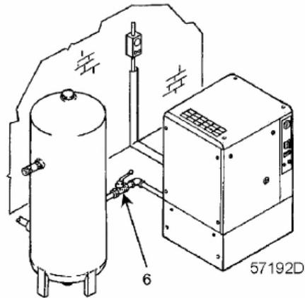
Installation proposal, Floor-mounted GX2 up to GX5
