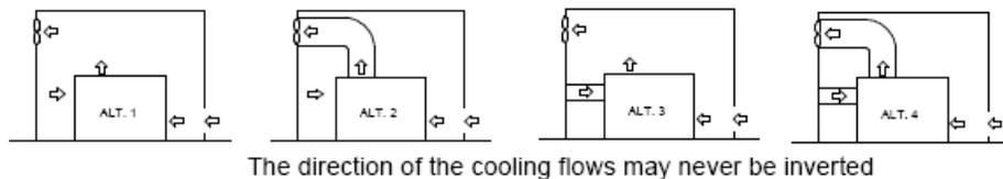
For alternatives 2 & 4 fan capacity should match the compressor fan capacity at a pressure head equal to the pressure drop across the cooling ducts.
