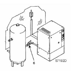
Installation proposal, Floor-mounted GX2 up to GX5
